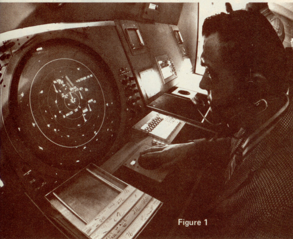
Figure 1—When the pilot is asked to "squawk Mode C," or "squawk altitude," his transponder transmits coded altitude information from his encoding altimeter to FAA's ground radar equipment. The altitude information is then decoded and automatically displayed on the controller's scope. Figure 2—this blowup of an Arts III alphanumeric information block shows the type of information that is automatically available to the controller. The aircraft shown is United Air Lines flight 789, squawking 6,900 feet msl, with a computed groundspeed of 170 knots. Univac photos
